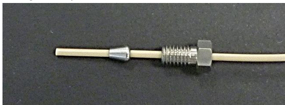
Figure 12. Assembly of stainless-steel nut and ferrule onto 1/16" OD PEEK tubing.
