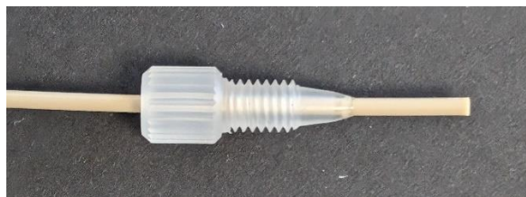
Figure 15. Assembly of a dedicated flow cell connector ('Fingertight fitting PCTFE 10-32', pn. 250.5171) onto a 1/16" OD PEEK tubing.
