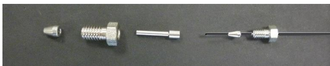
Figure 26. Exploded view of internal reducer (1/32" to 1/16") with the 1/16' nut and ferrule to the left, the 1/32' nut and ferrule mounted on the 1/32" OD PEEKSil tubing and the through-bore filler in the middle.
