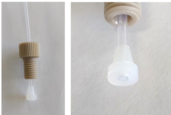
Figure 10. Assembly of 1/4-28 nut, ferrule (for connection in a flat bottom port), and 1/16" OD tubing for connection to SSV and degasser ports. Make sure to align the tubing end with the ferrule bottom (it should not protrude out).
