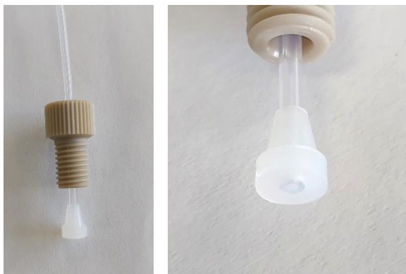
Figure 31. Assembly of 1/4-28 nut and dedicated ferrule for connection of 1/16" OD tubing in a flat bottom for 1/8" OD port.
