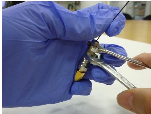
Figure 42. Connecting the 1/32" OD PEEKSil tubing to a prefilter with 1/16" receiving port requires holding the tubing into the bottom of the port while closing the nut with considerable force.
