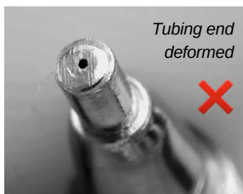
Figure 18. Sleeved SS tubing leaks and shows deformation after tightening the nut with the tubing end bottomed into the receiving port
