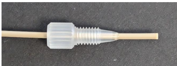
Figure 35. Assembly of a dedicated flow cell connector ('Fingertight fitting PCTFE 10-32', pn. 250.5171) onto a 1/16" OD PEEK tubing.
